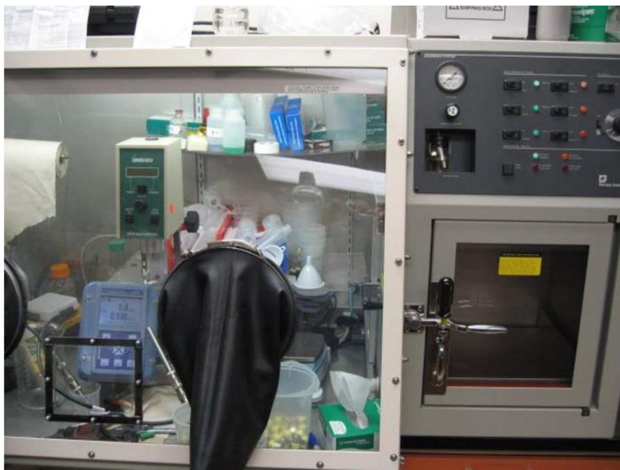
Fig. 1—Anaerobic chamber.
