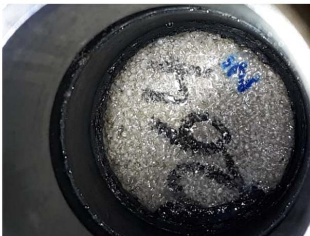
Fig. 5—SG1 gel on the injection face at the end of the coreflood.
